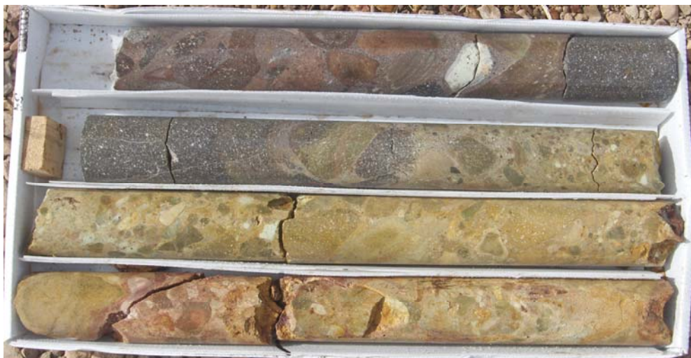
Figure 26: An Example of Selectively and Slightly Weathered / Leached Andesite Agglomerate of the LVS, in a Zone of Otherwise Massive, Fresh and Unweathered Material (drillhole BP10-673, 116.40 m to 118.65 m, top of section at top left) (taken during AMEC's January/February 2012 site visit)
