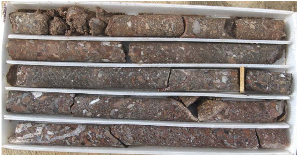
Figure 23: A Rare Example of Severe Local Weathering of Otherwise Intact and Fresh Breccio-Conglomerate, the Former as Marked by the Clay-Rich Material Near the Top of the Drillcore Section (drillhole BP08-266, 158.99 m to 161.88 m, top of section at top left) (taken during AMEC's January/February 2012 site visit)
