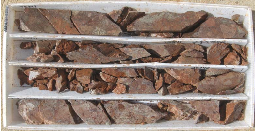
Figure 39: An Example of Extensive Drilling Damage to a Section of Slightly Altered (Hematite), Andesite Agglomerate Drillcore Affected by Steeply Inclined, Irregular Discontinuities, with Minor Limonite Infilling (drillhole BP08-211, 87.23 m to 89.27 m, top of section at top left)
