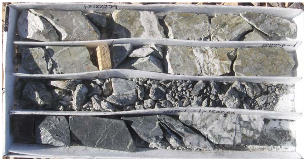
Figure 38A/B: An Example of an In-Box Degraded, Broad Zone of Occasionally Intense Propylitic Alteration Around the Schist-Sedimentary Nonconformable Contact
