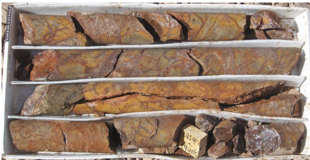
Figure 27: An Example of Selectively and Slightly Weathered / Leached Andesite Agglomerate of the LVS, in a Zone of Micro-Fracturing Associated with Hematite Alteration (drillhole BP10-560, 192.35 m to 194.35 m, top of section at top left) (taken during AMEC's January/February 2012 site visit)
