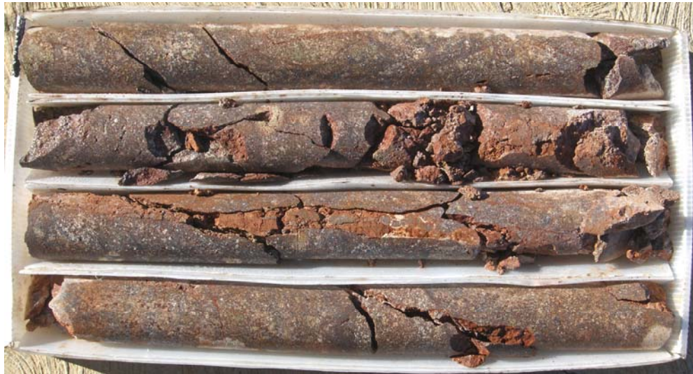
Figure 21: Sub-Vertical and Undulating Open Void Joint with Thick Limonite Infillings (drillhole BP08-254, 7.95 m to 10.16 m, top of section at top left) (taken during AMEC's January/February 2012 site visit)
