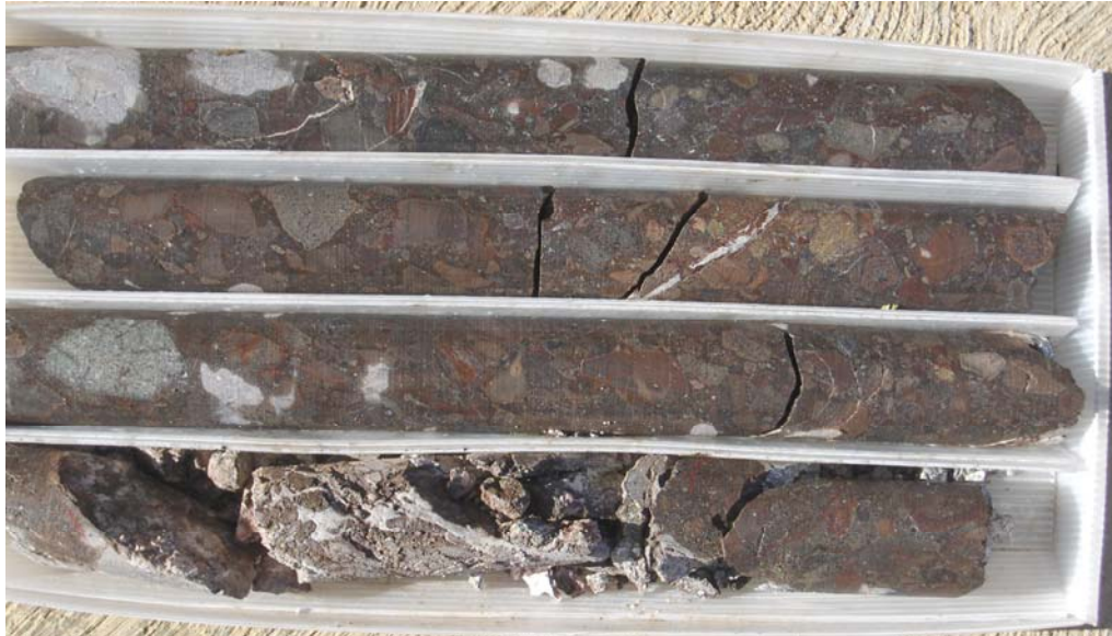
Figure 5: Coarse Crystalline Infillings in Open Void Structures in a Section of Weakly (hematite) Altered Andesite
