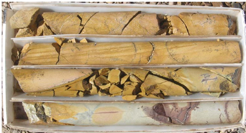
Figure 24: An Example of Local Weathering / Leaching of an Otherwise Intact and Fresh but Locally (hematite) Altered Andesite Tuff of the LVS (drillhole BP05-006, 105.70 m to 107.95 m, top of section at top left) (taken during AMEC's January/February 2012 site visit)
