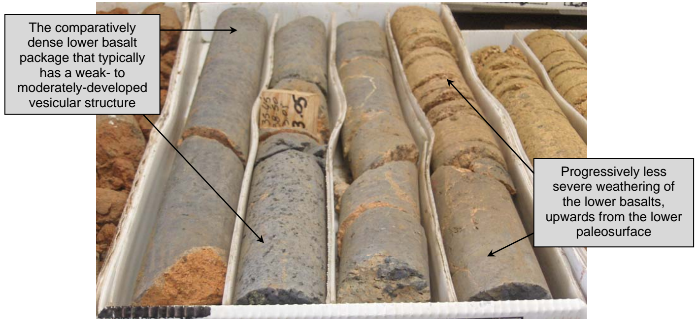
Figure 12B: 37.65 m – 39.80 m (boxes 2 to 16 missing – basalt sequence only)
