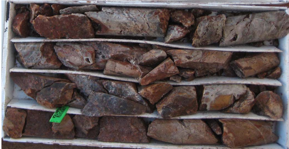
Figure 20: An Example of Extensively Drilling-Damaged Vein Material, due to the Presence of Minor Vugs and, Most Importantly, Sub-Vertical, Open Joints (drillhole BP10-467, 121.80 m to 123.95 m) (taken in 2010, shortly after the hole was drilled, photolog supplied by Pan American)
