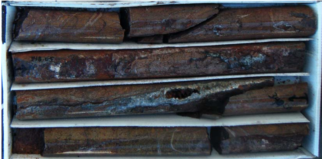
Figure 7: An Example of a Steeply Inclined, Undulating and Rough, Unmineralized but Limonite-Stained, Open Joint in Association with a Silicified Vein Intersection and a Hematite-Altered and Slightly Weathered / Leached Andesite
