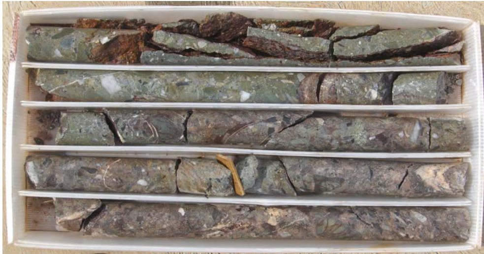
Figure 22: Sub-Vertical and Undulating Open Void Joint with Minor Limonite Infilling (drillhole BP08-266, 320.26 m to 323.01 m, top of section at top left) (taken during AMEC's January/February 2012 site visit)
